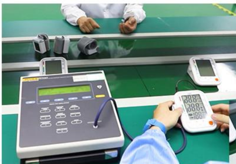
Blood pressure monitor simulation detection this is the most importance step to ensure the accuracy
